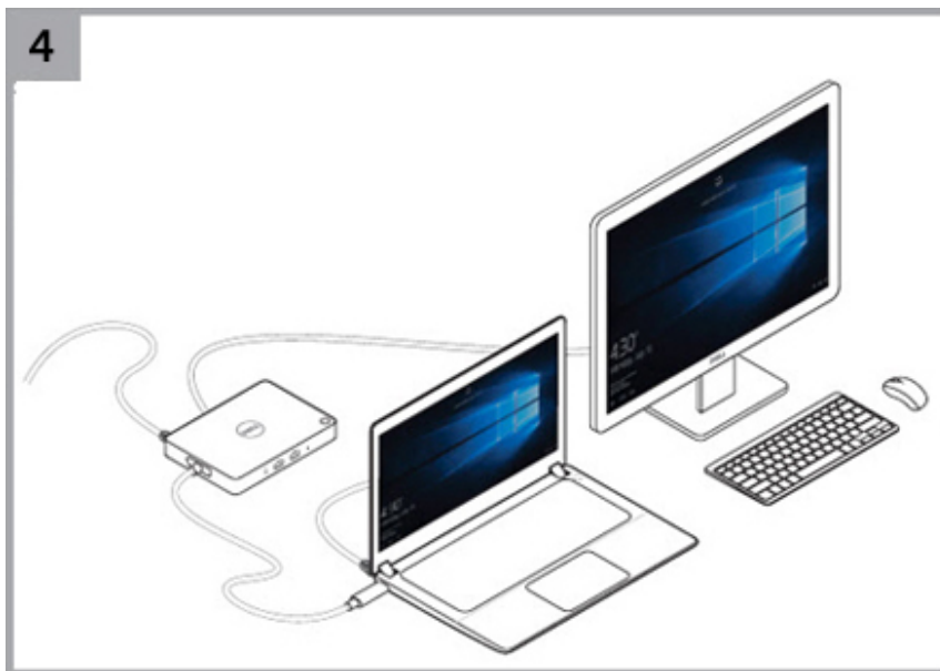
Figure 5. Connecting the USB Type-C connector
